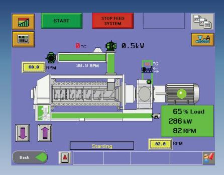
Compress V is a PLC based control system designed specifically for the control and optimisation of a screw press. It can be extended to control an associated vertical type Stack cooker and is available not only for the Sterling Series, but almost any screw press.
