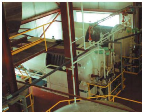
The mass of oil is gradually cooled by means of glycol water circulating inside cooling coils. One or several coolers are installed according to plant capacity. The oil overflows continuous from one to the next series.
