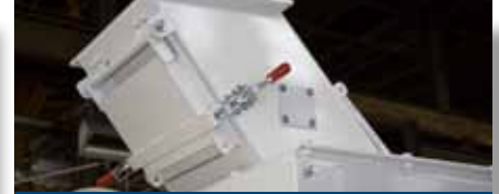
Magnet on feed chute
