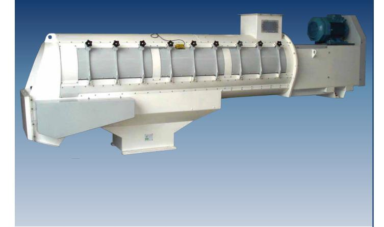
The long residence time horizontal conditioner purpose is to increase the residence time of the heated meal and improve the parameters required to obtain a high quality pelleting results. The processing temperatures range from 60°C to 100°C for a treatment time of 30 seconds up to 6 minutes.
