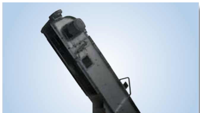
Curved chain conveyor head
