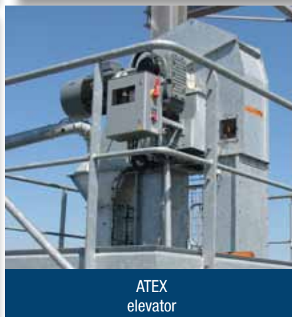
High capacity elevator head (1600 m 3 /h, height 65 m, 2x200 kW)
