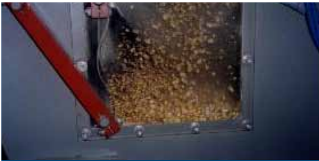
Adjustable flap for air/product segregation
