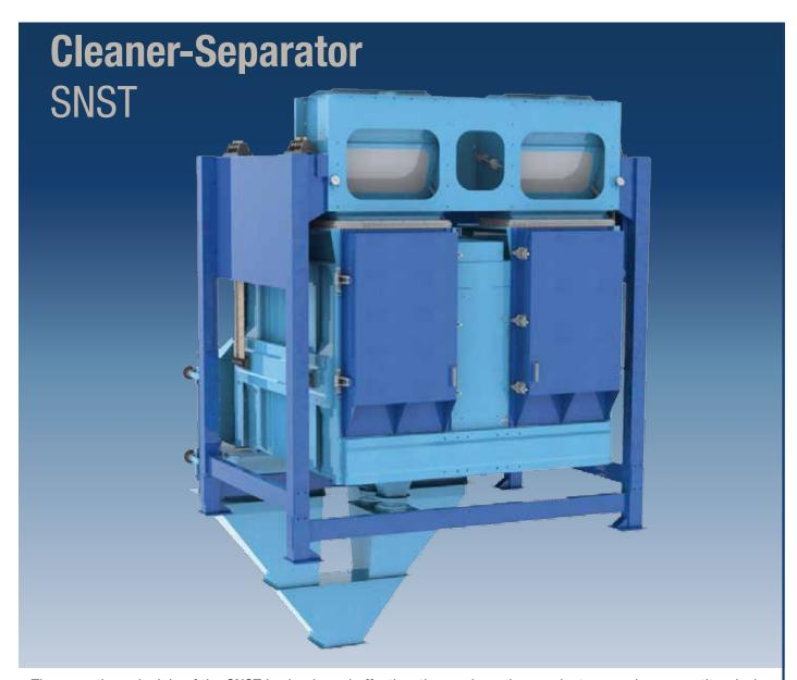
The operating principle of the SNST is simple and effective, the seed or other product comes by a repartitor device on the total width of the first screen. The efficacity of the screening is increased in important proportions by weighted rubber balls to insure the cleaning of the whole working surface, without the wear of the grids.
