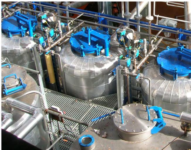
De Smet has developed an enzymatic interesterification technology, called Interzym, in collaboration with the company Novozymes (Denmark). Enzymatic interesterification is an efficient way of controlling the melting characteristics of edible oils and fats.
