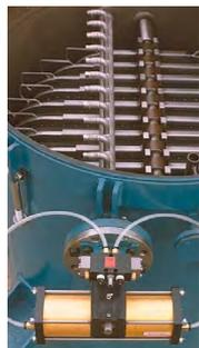
for about 30 min to remove as much water as possible. During drying, the oil is pumped around in order to speed up the drying process.
